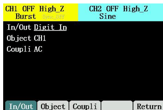
Figure 2-35 multiplex port interface input setting
